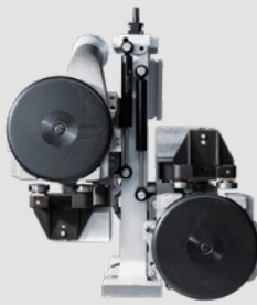
MF21 multi-trimming unit
