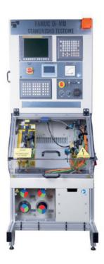
The photo shows a test bench for FANUC 0i- MD.
