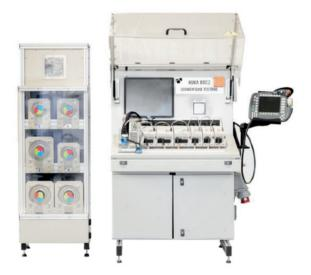
The photo shows a test bench for KUKA KRC2.
