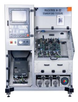
The photo shows a test bench for Mazatrol M-32 Mitsubishi.
