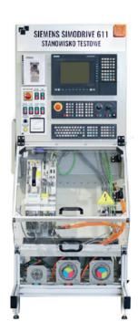
The photo shows a test bench for Siemens Simodrive 611. Our offer also includes test benches for Siemens 611 High performance.
